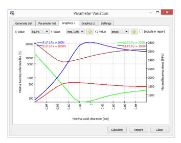
depending on the moment load, but also which axial clearance brings down the contact pressure, pmax, to a minimum value.
