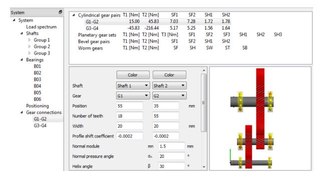
The torque on each gear pair is shown in the list at the top; the safety factors are shown if a connection to a gear calculation program is set up.
