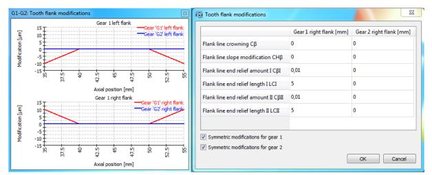
All in all, the user can make use of the line load and gap width graphics as guidance to stablish a flank correction proposal. If, for instance we start from a gear tooth mesh condition like this:
