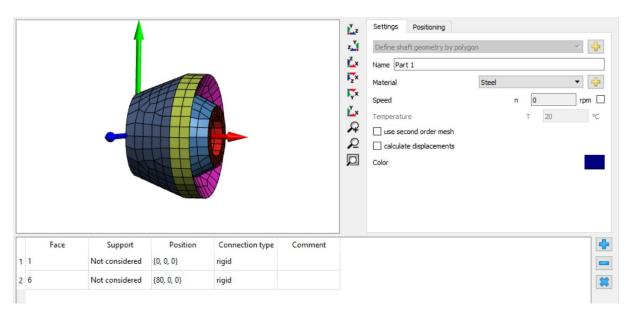
Using the +-button behind "Define shaft geometry by polygon" a dialog opens to define the geometry using a polygon. It should be defined clockwise. "x" is the axial coordinate, "y" the radius. Optional connections to normal shafts can be defined as "Considered as face" or "Considered as edge". Either all points on a face or only points on an edge will be connected to a shaft support element.
