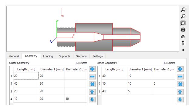
There is an input table for both inner and outer geometry. The plus- and minus-buttons allow adding and removing rows, the arrows can be used to move an element up or down in the table.
