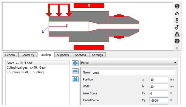
Loads can be added by the plus button next to the list. The type of the loading can be selected using the list on the right. Each load element has a name to identify it, a position relative to the left end of the shaft and a width.
