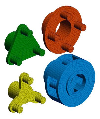
For an imported planet carrier, the rotation axis has to be the x-axis.
